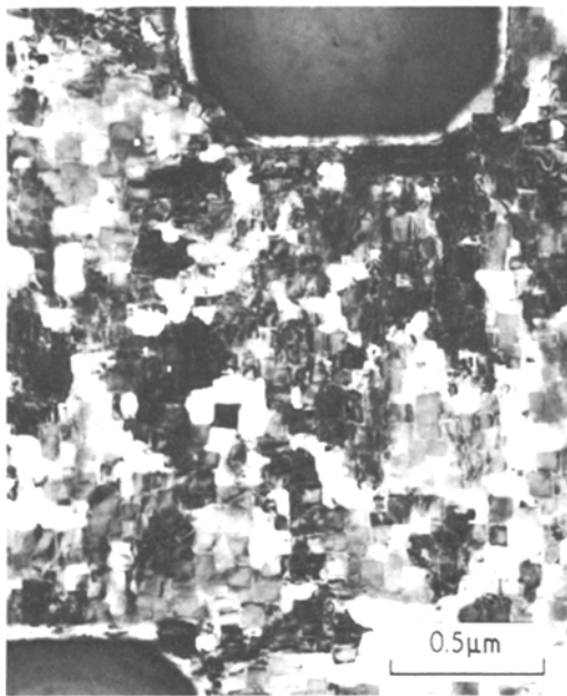
Figure 2 TEM from a transverse section of the eutectic water-quenched from 1260°C, well above the \gamma' solvus temperature, showing a configurational change of \gamma' from blocky to fine cuboidal shape (cf. Fig. 1b).
